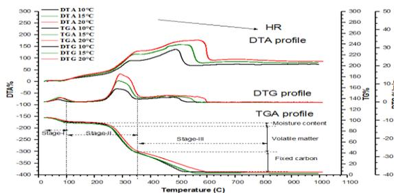
Figure 1. Thermal degradation of pearl millet cob
