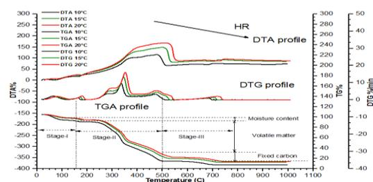
Figure 2. Thermal degradation of eucalyptus wood
